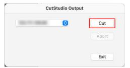
The cut data is sent to the machine. When the machine receives the data, it automatically reads the crop marks using a sensor, and then starts cutting.
