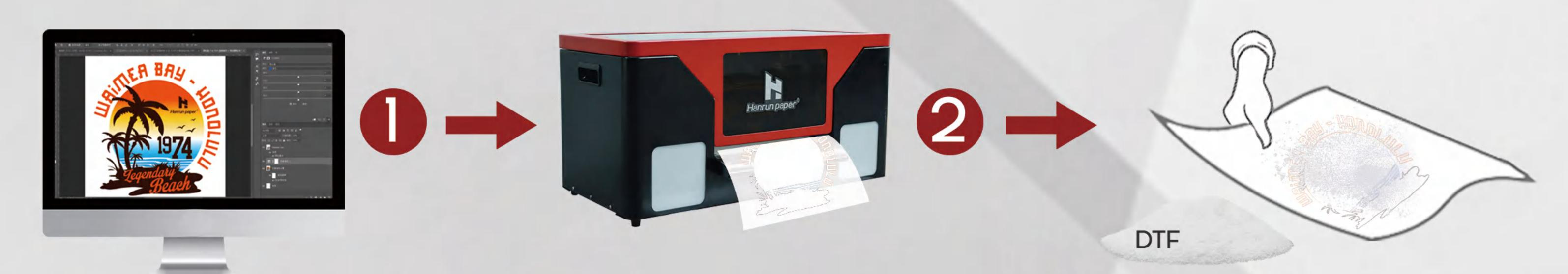
1. Computer design (15-20 seconds) 2. Printed the image with DK A-30 DTF PRINT-ER (5-8 mins)
